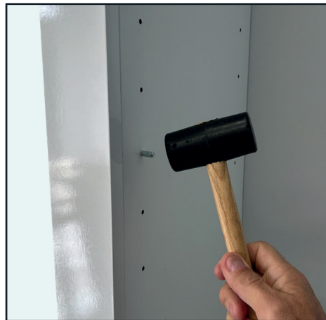
5. Insert all shelf supports into holes at the desired heights.
